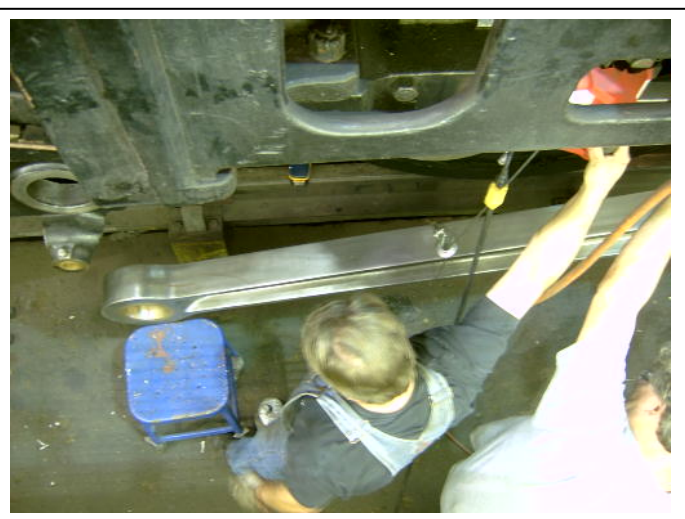
The left main rod was finally installed. We lowered it down to where it is with the use of the overhead crane. While it was hanging from the crane, the other end of the rod, the big end, was fitted to the crank pin. Then the small end, the visible end in the photo, was set down by the overhead crane and picked up with the portable winch that can be seen hanging if one looks closely. This picked the small end of the main rod up and it could be brought into place so the wrist pin could be shoved through. That part fell to me. Steve said, "Ok, we need a man to get under there and lift the wrist pin into place, who's going to do it?" I said, "Well, being the only man here, I guess it's me." And so it was. I need to learn to keep my big mouth shut.' It weighs about 75 pounds and has to be lifted above my head and then pushed through the hole. Not tough, really, but I like to complain.
