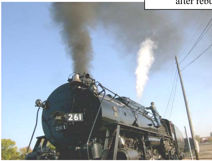
Setting the Pop's. Otherwise referred to as safety valves or safeties. The boiler was designed with a safety factor of 7. I learned this during the time when all steam locomotive boilers had to have new certifications to meet new safety standards. Comforting to know, but it never runs over 250 psi anyway.
